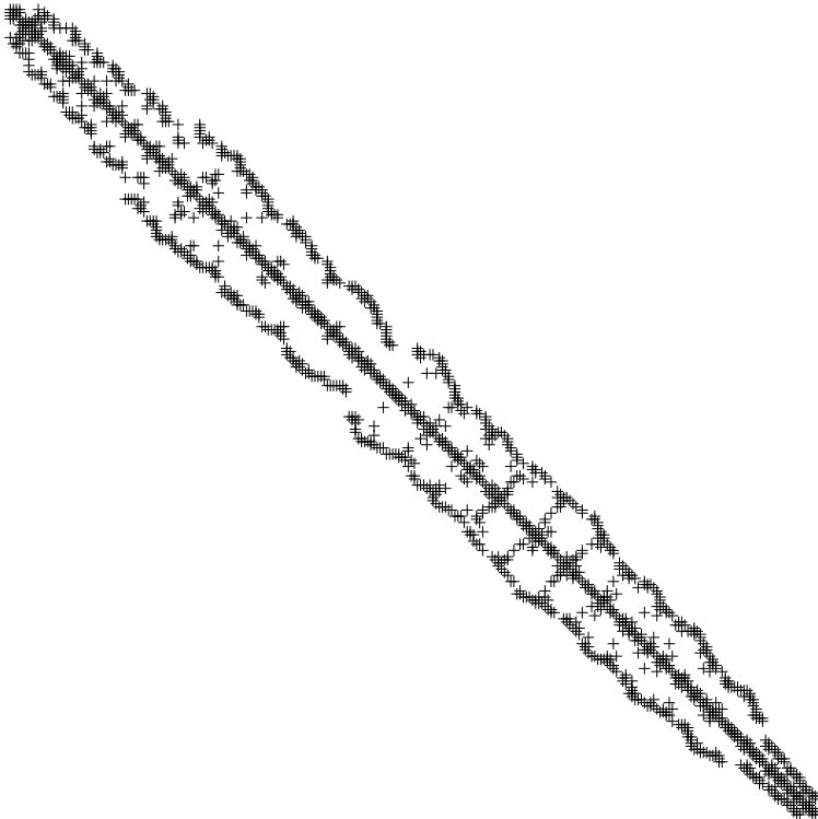
Figure 3: Sparsity of the FE Matrix After Renumbering
